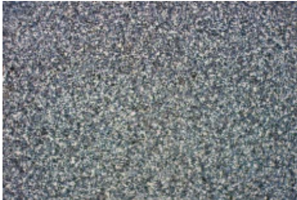
Fig. 6. Microstructure obtained after the normalisation treatment for the steel 40VMoCr11-ferite+fine perlite (x100)
