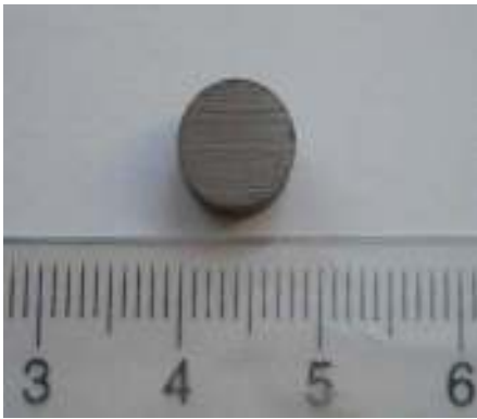
Fig. 4. Aspect of worn surface after the abrasion test
