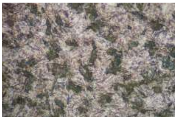
Fig. 13. Microstructure obtained after the quenching treatment for the steel 42MoCr11- white martensite + rezidual austenite + troostite (X500)
