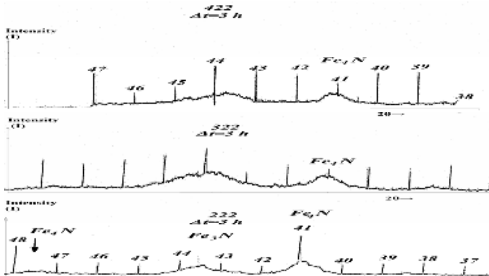
Fig. 5. Diffractometry aspects for: 222 samples ( T_1, Q=150 daN, \xi=10\% ), 322 samples ( T_1, Q=150 daN, \xi=20\% ), 422 samples ( T_1, Q=190 daN, \xi=20\% )
