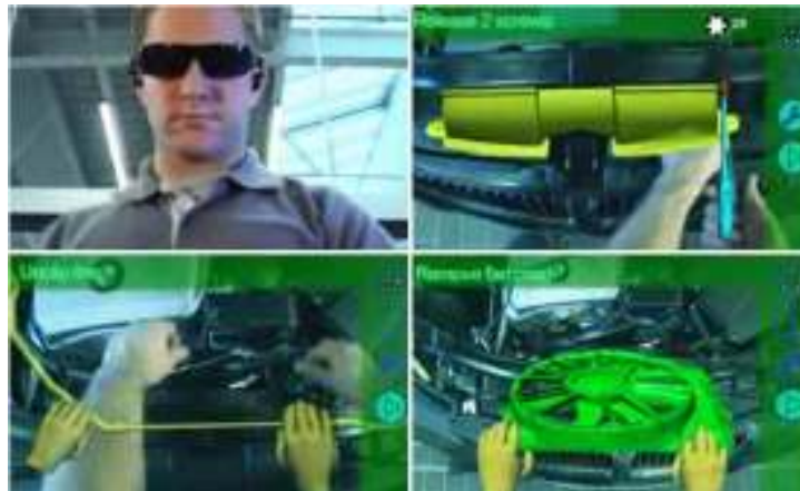
Fig. 1. AR application developed by BMW for workshop repair
