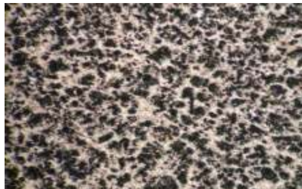
Fig. 11. Microstructure obtained after the quenching treatment for the steel 42MoCr11- white martensite + rezidual austenite + troostite (X100)
