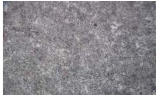
Fig. 9. Microstructure obtained after the normalisation treatment for the steel 42MoCr11-ferite+perlite (X500)
