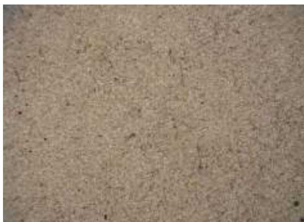
Fig. 14. Microstructure obtained after the quenching + high annealing treatment (improvement) for the steel 40VMoCr11- sorbite (X100)
