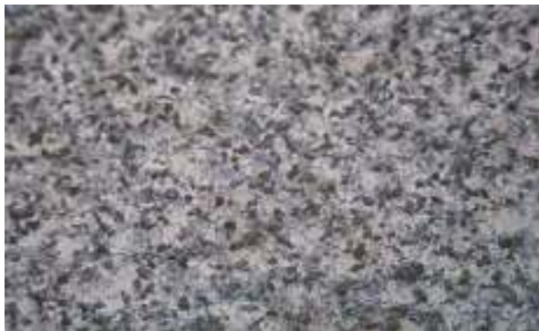
Fig. 8. Microstructure obtained after the normalisation treatment for the steel 40VMoCr11-ferite+very fine perlite+ troostite (x500)
