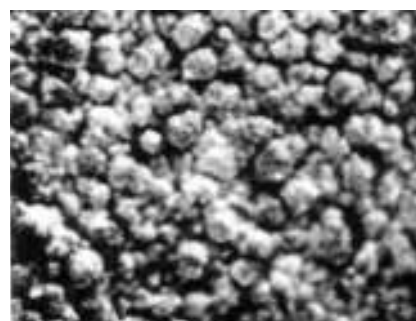
Fig. 2. Co/ferro-niobium composite layers; current density: 570A/m 2 ; 50X
