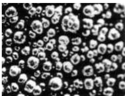
Fig. 1. Cobalt layer; current density: 570A/m 2 ; 50X
