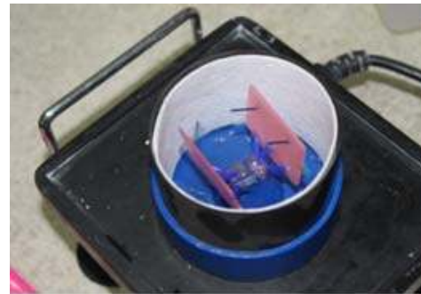
Fig. 4. Layout models as a whole form-fitted models on the table vibrating, ready pentru turnarea mass packaging
