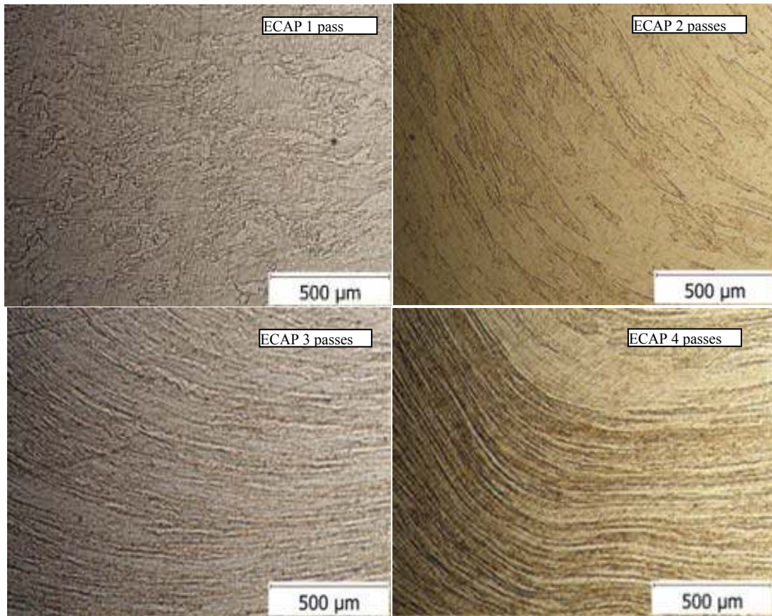
Fig. 7. OM of ECAP billets Region B after one pass (a), 2 passes (b), 3 passes (c), 4 passes (d),
