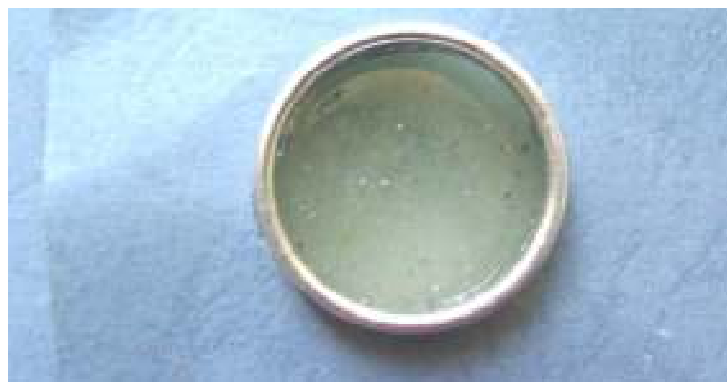
Fig. 3. Glass with nickel oxide after thermal treatment
