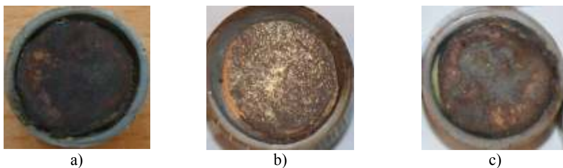
Fig. 8. The electrode surfaces after the corrosion test performed in a solution containing 0.2g/L \text{Na}_2\text{SO}_4 + 0.2g/L \text{NaHCO}_3 (pH = 5), a) patina 1, b) patina 2, c) patina 3
