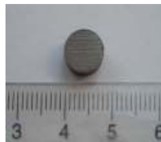
Fig. 3. Worn surface after the abrasion test
