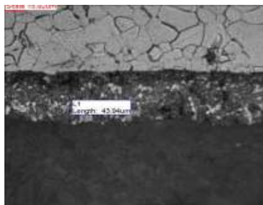
Fig. 5. microstructure of the 32%Sn-68% Pb alloy coating immersion duration: 9 seconds, temperature 185[°C]
