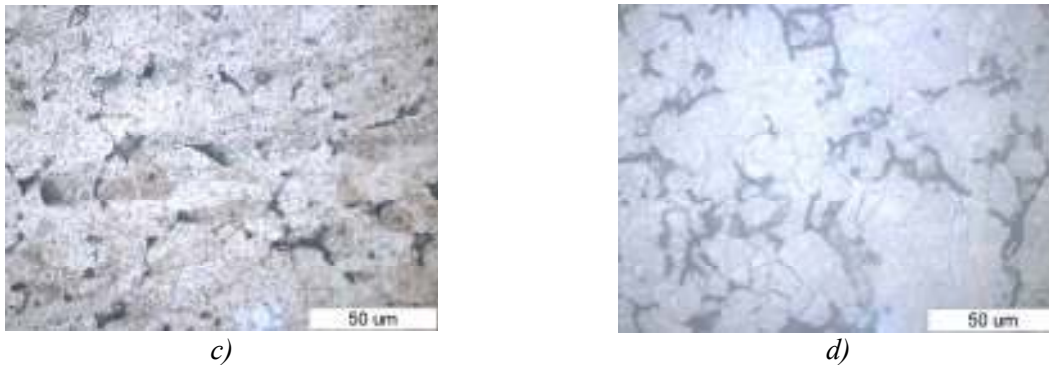
Fig. 4. Microstructures of 316L stainless steel samples compacted at pressure of 600 MPa: a) classical compaction of 6.5 g samples, b) with friction assisted compaction of 6.5 g samples, c) classic compaction samples of 10.5 g d) compaction with friction assisted samples 10.5 gr.
