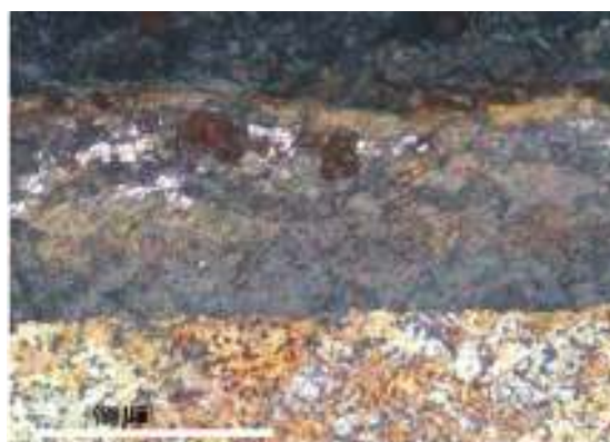
Fig. 9. Microstructure of bronze-steel bimetal after 3 week exposure to sea water [26].
