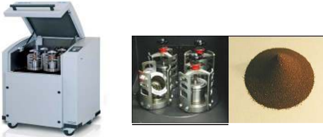
Fig. 3. Retschmaschine and steel vials for preparing mixed powder of Cu7Ag 0.05Nb for compressed rods.
