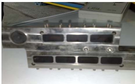
Fig.2. Head transducers, seven unfocused transducers (rectangular) and a focused transducer (circular shape)
