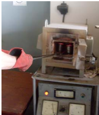
Fig. 2. Furnace used for melting the bronze chips into the steel support
