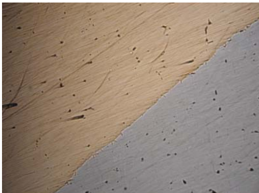
Fig. 7. Aspect of bimetal at interface (100X without exposure to metallographic attack)
