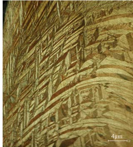
Fig. 7. Optical microstructures CuAl 13 Ni 4 alloy after ausforming with 20% deformation degree, from 800°C. Curved martensite
