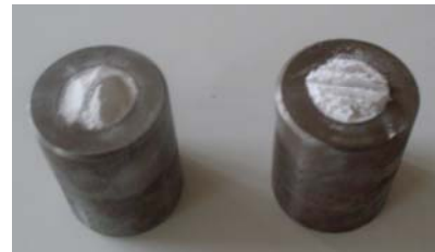
Fig. 4. Preparation of the samples before insertion in the heating furnace
