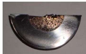
Fig. 5. Bronze chips incompletely melted often being heated at 1200^\circ\text{C}
