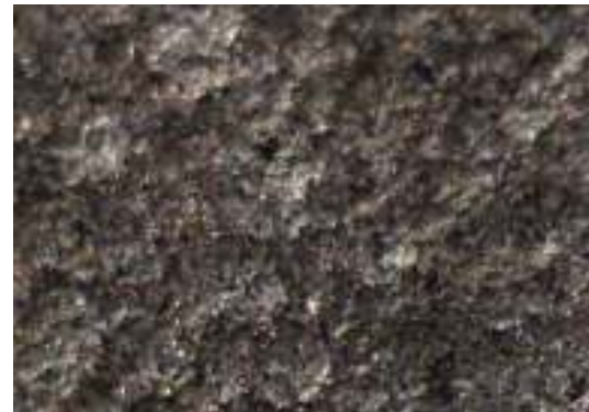
Fig. 10. Macrostructure photograph obtained with oil medium deposition method, two layers
