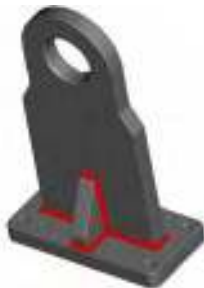
Fig. 8. Support made of welded semi-products.
