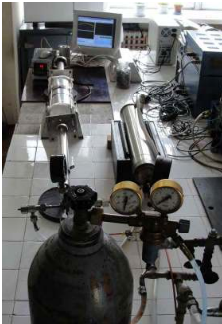
Fig. 1. Installation for producing TiH 2 .
