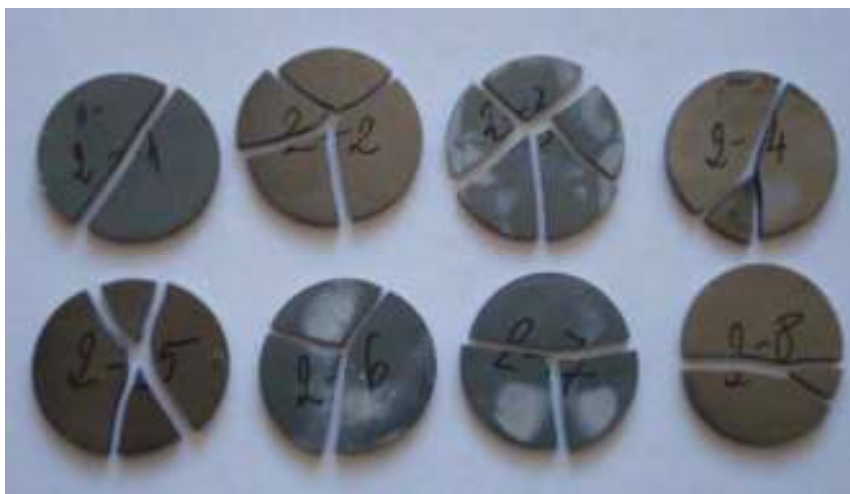
Fig.6. Specimens from reinforced titanium ceramic – type 2 after fracture.
