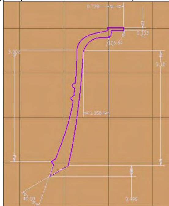
Fig. 2. Bell shape and size obtained by Autodesk.
