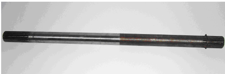
Fig. 1. Construction of real input shaft from the reducer about rope electric hoist.
