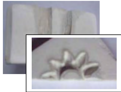
Fig. 7. Section in the mould ready for casting.
