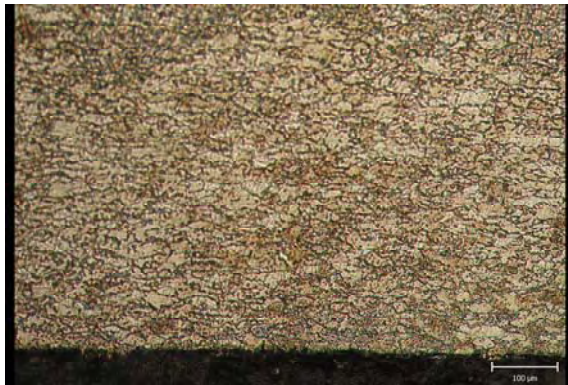
Fig.12. Micro-structure of material in the frontal wall of the stamped part (Nital 5).
