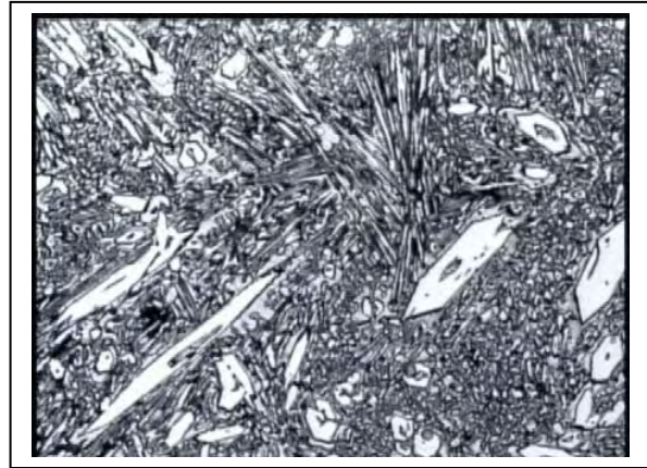
Fig. 4. Variant C, layer structure, martensite and coarse acicular carbide x200.
