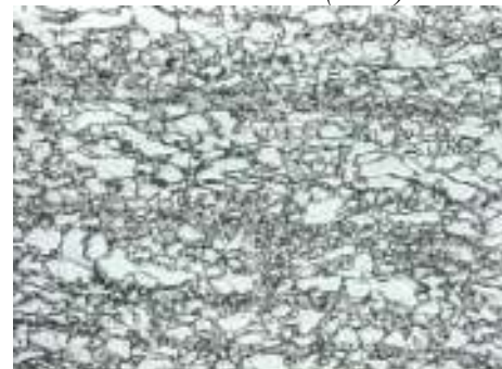
Fig. 8. Intercritical thermomechanical treatment state - D variant (x500).
