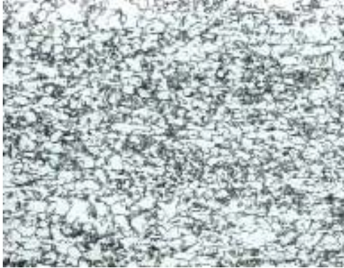
Fig.9. Intercritical thermomechanical treatment state - G variant (x500).
