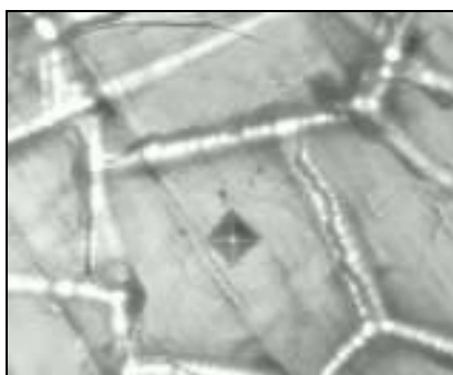
Fig. 5. Indentation hardness in electrodeposited Ni films on Cu substrate at i = 3.333 \text{ (A/dm}^2\text{)} , T = 30 \text{ }^\circ\text{C} and \text{pH} = 6.21
