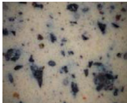
Fig.4. BF dust particles with varied shapes (polyhedral shapes and rounded)
