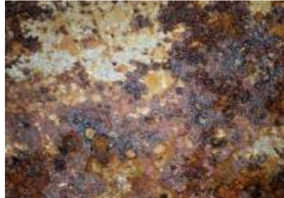
Fig. 7. The macrostructural aspects of the steel sample surface exposed to corrosion, after 112 days of natural ageing, \times 100
