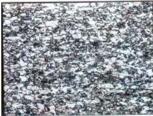
Fig.10. Intercritical thermomechanical treatment state - I variant (x500).
