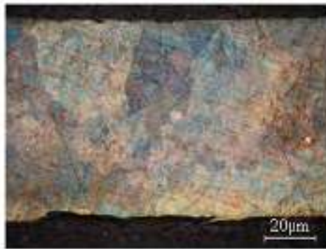
Fig3. Microstructures of hot rolled alloy at 30% deformation degree and 950 o C
