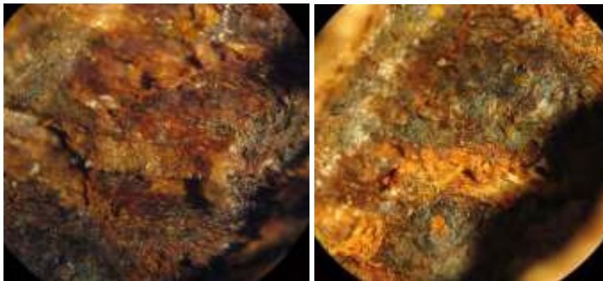
Fig. 5. Images taken with optical microscope of wood with iron traces non-uniformly distributed
