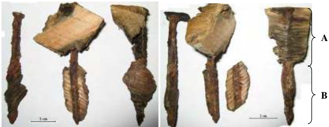
Fig. 4. Longitudinal section of the wood-metal interaction area: A – the floor; b – joist
