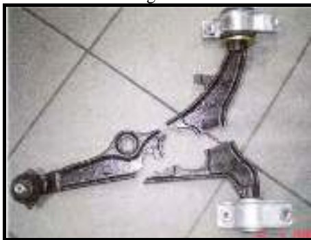
Fig.1. „Arm – wheel support” - cracked piece.
