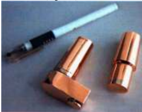
Fig. 8. Appearance of contacts for vacuum blowout chambers
