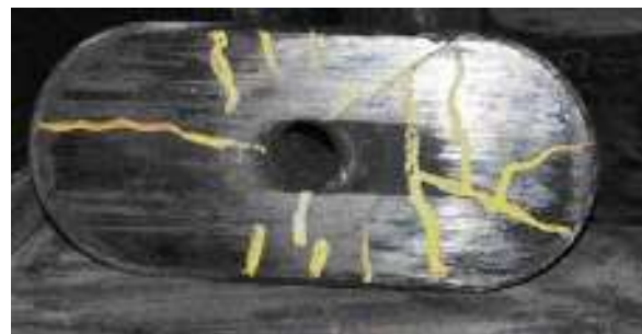
Fig.1. Rectangular-rounded plate with cracks
