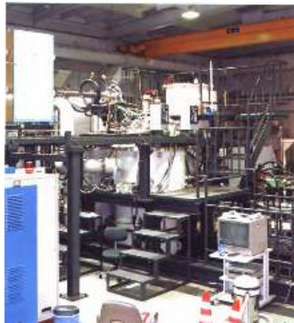
Fig. 10. 500 kW electron beam unit for silicon remelting
