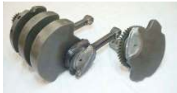
Fig. 2. Crankshaft and engine piston broken by mechanical fatigue [Minho Univ.].
