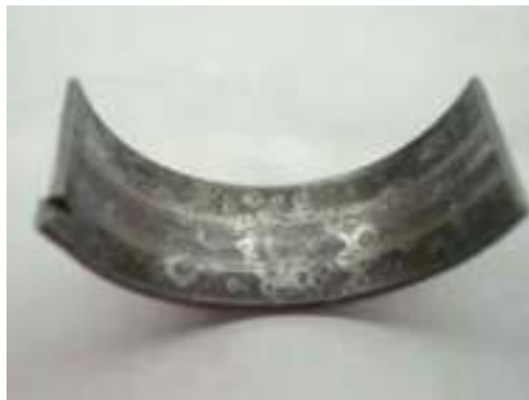
Fig. 14. Journal bearing damaged by abrasion fatigue [Minho Univ.].
