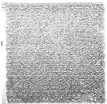
Fig.7. Surface macrograph for sample no.7 700V/ 7,5mm/ 0,3Hz). Magnitude 5x.
