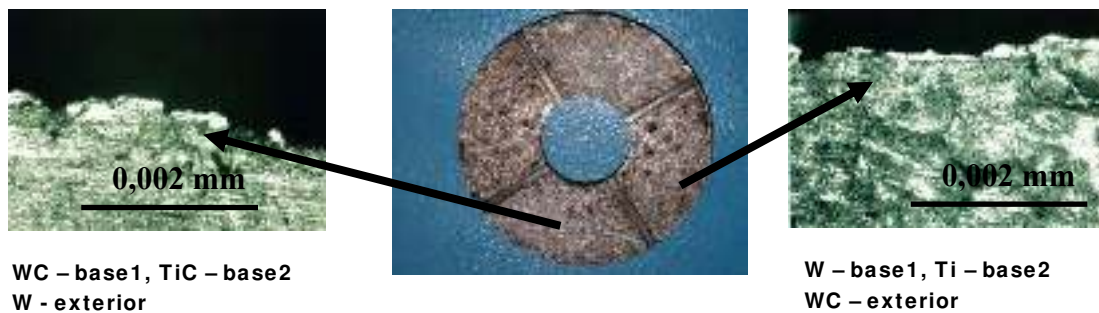
Fig.4. Cast iron sample with different kind of deposition-macrostructure; Microstructure triple layer deposition, first layer W, second layer Ti, WC exterior layer and WC first layer, TiC front layer, W exterior layer
