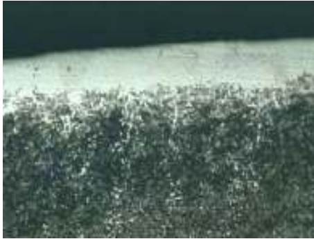
Fig. 6. Nitrocarburized layer on the sample R5 (code R), before wear process tests.
