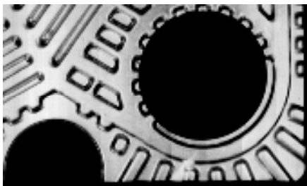
Fig. 5. Uncracked area of the heat exchanger
