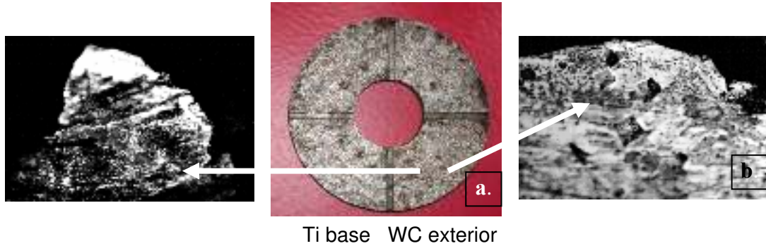
Fig.3. a. Cast iron sample with different kind of deposition-macrostructure; b. Microstructure double layer deposition, first layer Ti deposition and front layer.
