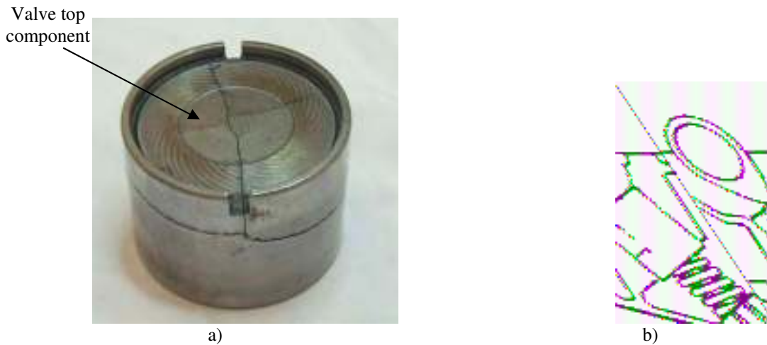
Fig. 8. a) Valve top component damaged by impact fatigue [Minho Univ.]; b) Working positioning of valve top component.
