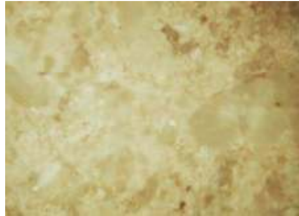
Fig. 5. The exterior of the refractory wall ( t = 100\text{ }^{\circ}\text{C} ; time = approx. 4 months)
