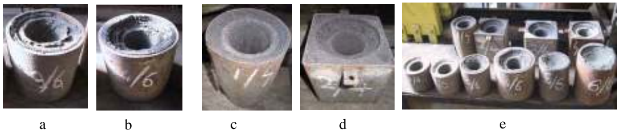
Fig. 3. a, b - Sample with dross and furan resin; c, d -. Sample with dross and soda water glass and Fortera; e- Samples after 48 hours
