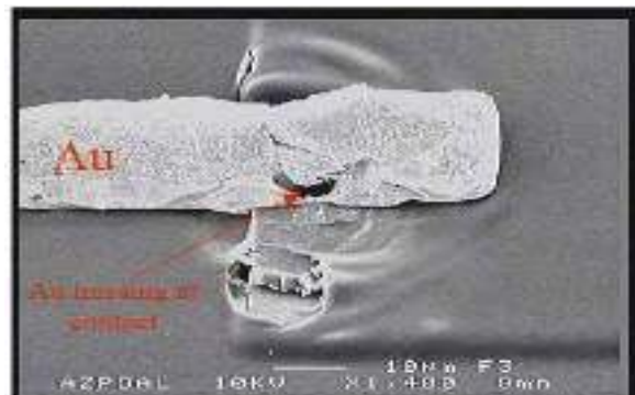
Figure 5. Power Au line with void above contact to aluminum after extremely high temperature testing and 860mA current. Gold diffused into aluminum and left a void.
