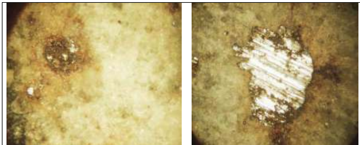
Fig. 1. Lining – melt metal interface ( t = 1450 °C; time = approx. 4 months)
