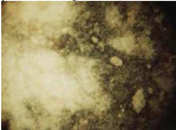
Fig. 2. = 10 mm from the lining – melt metal interface ( t < 1450\text{ }^{\circ}\text{C} ; time = approx. 4 months)
