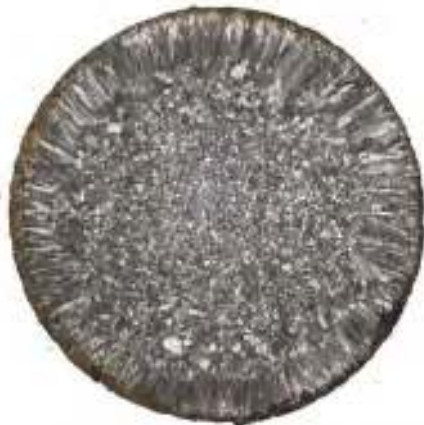
Fig.1. Unmodified steel macrostructure with 4%Si. Columnar crystals area is highlighted
