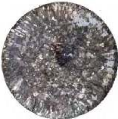
Fig.2. Unmodified steel macrostructure with 7.07%Si. Columnar crystals area is seen. Also, cracks are observed.
