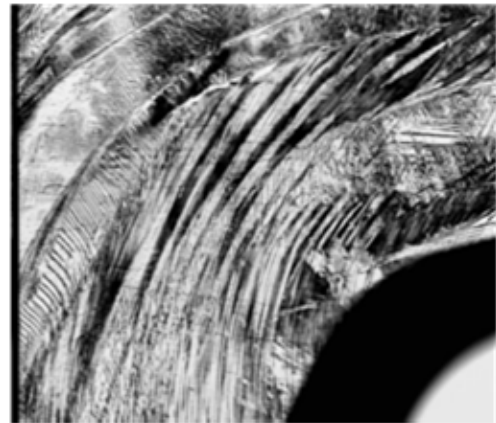
Smart memory alloy deformation degree 111% Chemical composition 12.88%Al, 3.84% Ni, rest Cu Microstructure: \gamma_1' Magnification: 100x
