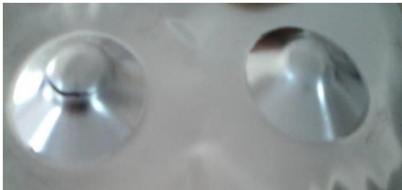
Fig. 4. Macroscopic aspect of Erichsen deformation
