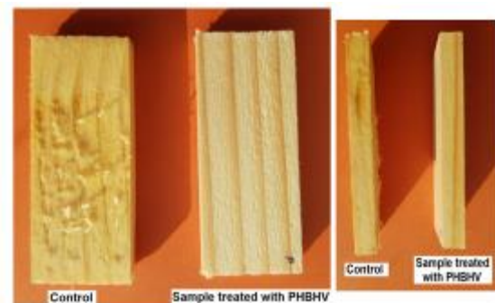
Fig. 6. The aspect of the samples after water absorption test (24 hours in water)
