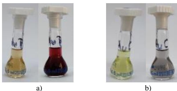
Fig. 2. Color changed after 4 and 24 hours of A) AuNP-AB and B) AuNP-AC solutions
