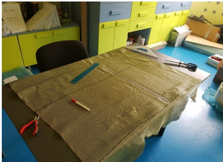
Fig. 3. Cutting high-density carbon-Kevlar fabric at different sizes
