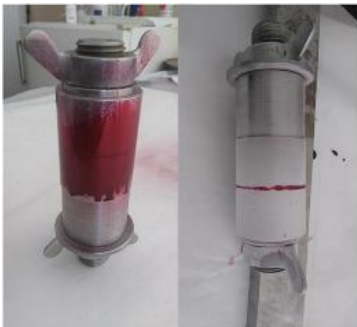
Fig. 2. Penetrant testing of the Miller etalon
