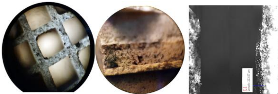
Fig. 9. Microscopic analysis of DPF channels after experimental tests for B30
