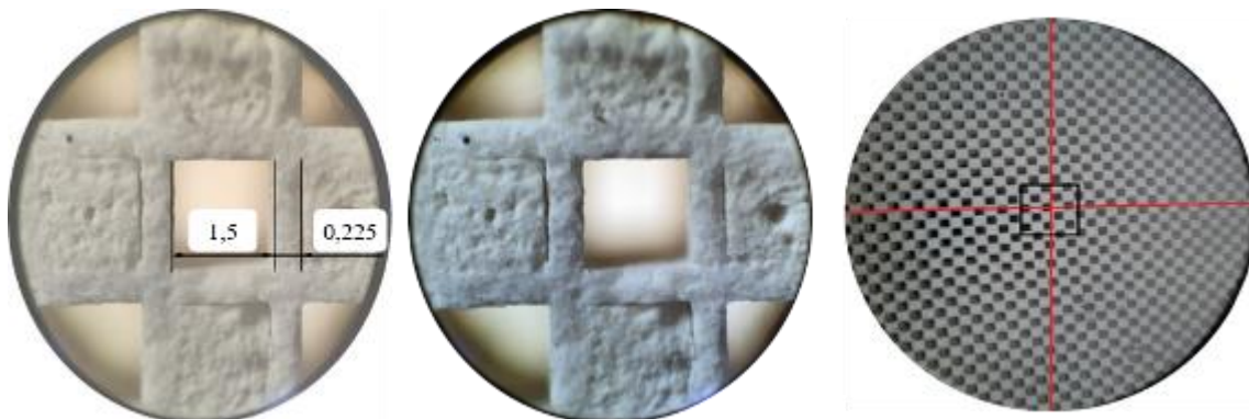
Fig. 6. Filter channels before the experimental tests and the area chosen for the microscopic study
