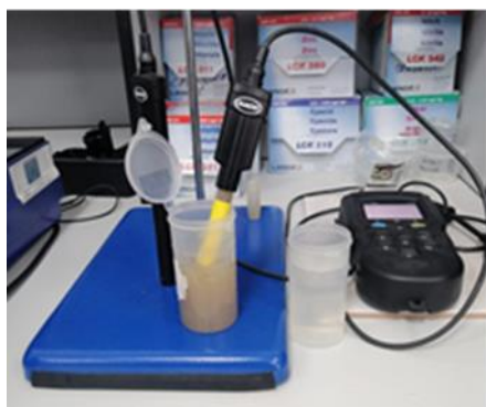
Fig. 3. PH measurement with soil-water suspension sample
