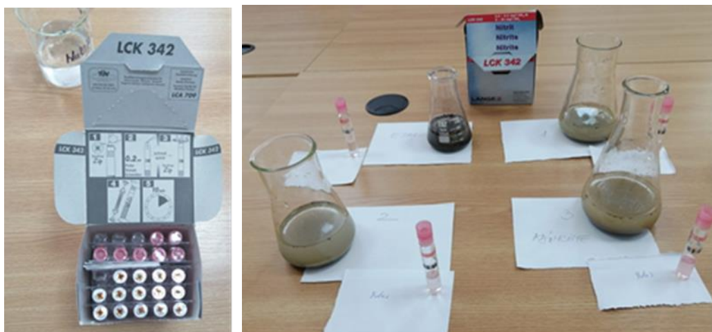
Fig. 7. Predetermined reagents LCK 342 for nitrite determinations
