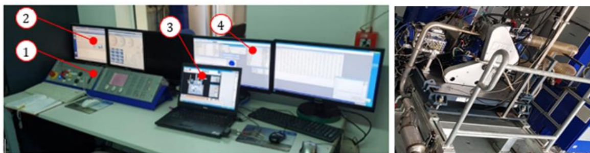
Fig. 2. Command chamber and AVL5402 engine used in experimental tests
