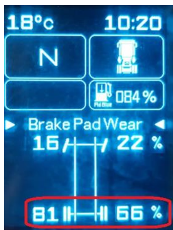
Fig. 1. Information provided to the user regarding the stage of wear of the brake pads
