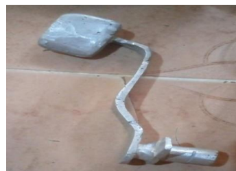
Fig. 15. After removing the excess material from the cast specimens (machined casts)
