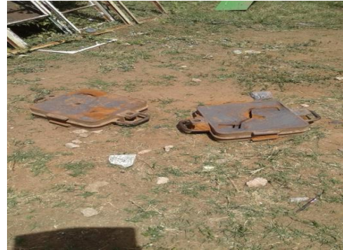
Fig. 10. The cope and drag after removal of patterns
