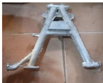
Fig. 14. The cast specimens before machining
