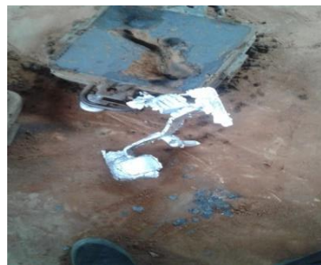
Fig. 14. The cast specimens before machining
