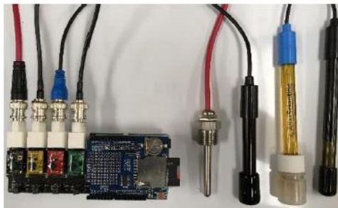
Fig. 8. The open-source multiprobe meter (OSMM) components [13]
