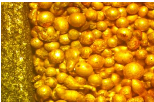
Fig. 2.2. The graphite mould with the powder prepared for sintering
