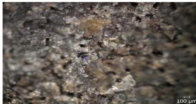
Fig. 4. The appearance of the sample, in the area at the shotcrete-refractory concrete interface
