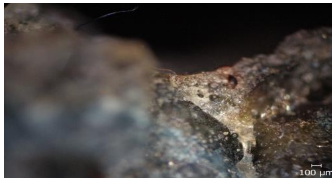
Fig. 3. Penetration of the liquid alloy into the capillaries of the ceramic material
