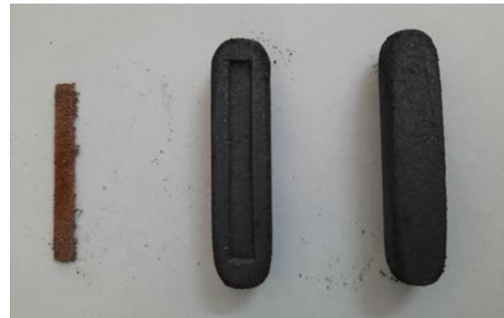
Fig. 2.5. Appearance of a sintered sample and the mould used for it
