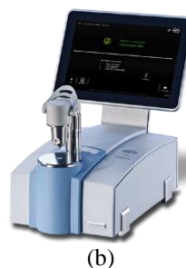
Fig. 1. Chitosan 'samples (a) and Bruker Alpha-P ATR FTIR equipment (b)
