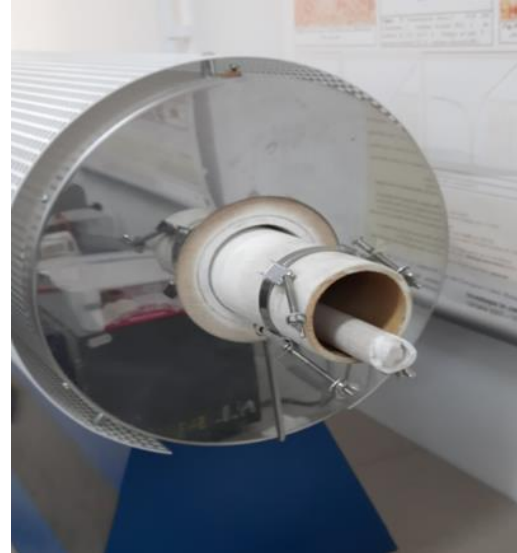
Fig. 2.3. The furnace used for sintering and the aluminium tube (to maintain the reducing environment), plugged with ceramic felt plugs, which contains the graphite form
