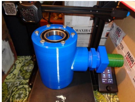
Fig. 1. 3D printed FA100 washing head housing at the end of PETG Material, assembled together with the other 3D printed parts of the FA100 washing head
