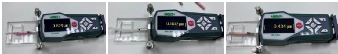
Fig. 8. Results of the roughness testing: K material sample – left image; M material sample – middle image; G material sample – right image
