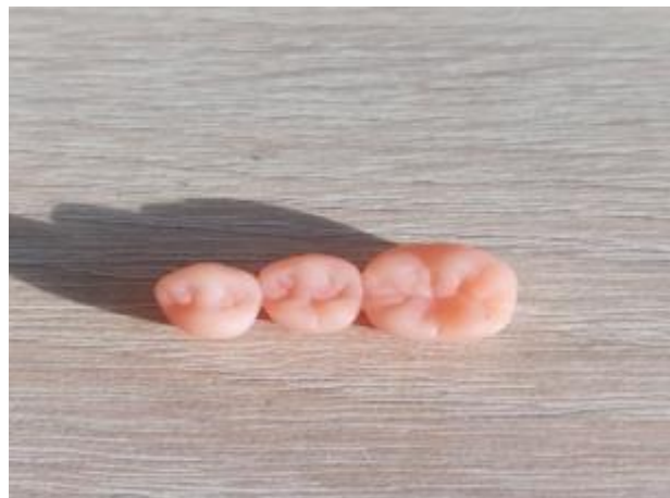
Fig. 10. The final dental bridge model, made of photopolymer resin, using SLA technology
