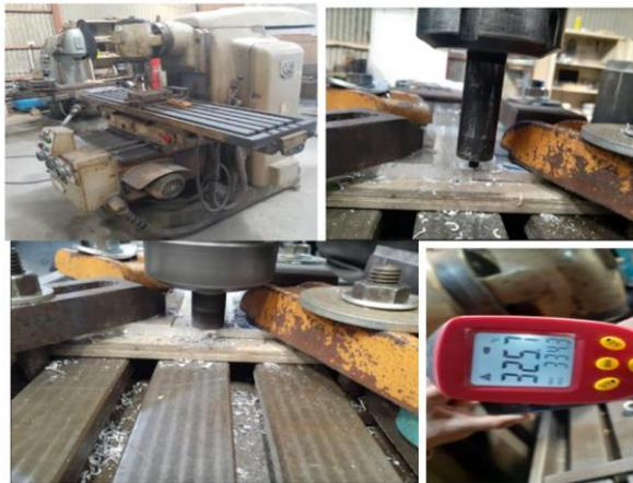
**Fig. 1.** Milling machine used in the friction stir welding
