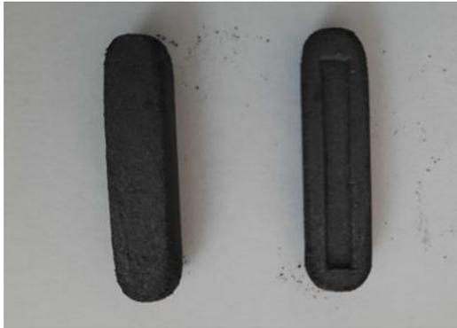
**Fig. 2.** The mould with the two semi-cylindrical components used for the free casting of CuSn12 powder samples
