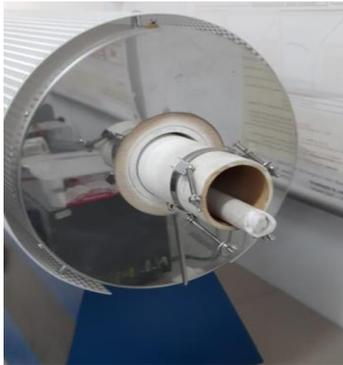
**Fig. 5.** The furnace LENTON used for sintering
