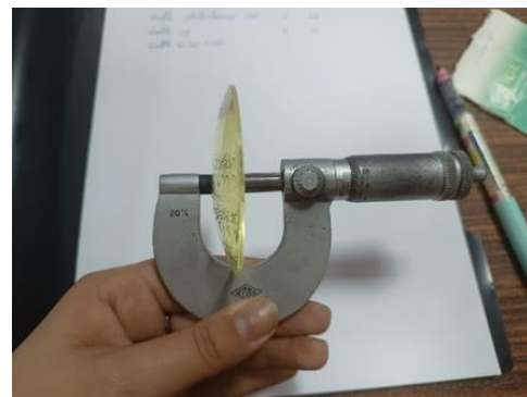
Fig. 2. Measuring lens thickness
