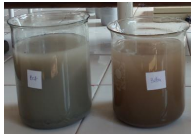
Fig. 5. The construction materials in contact for 24 hours at L/S = 10 L/kg
