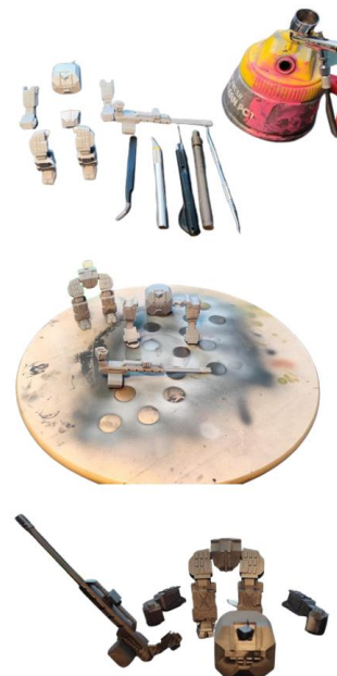
Fig. 5. Components painted with different coloured layers using an airbrush
