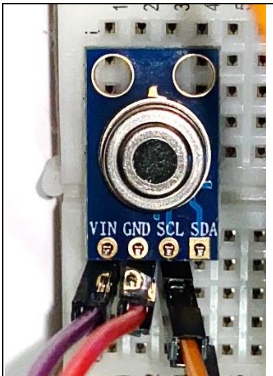
Fig. 2. The MLX90614 sensor pin connections
