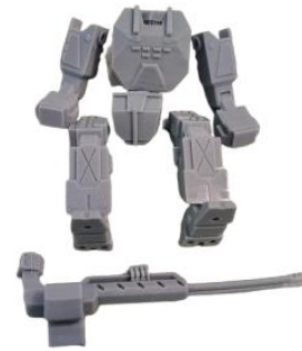
Fig. 4. Components printed using SLA technology
