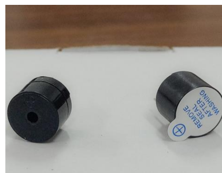
Fig. 5. Piezoelectric buzzer used for user alerts
