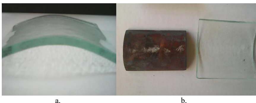
Fig. 11. Thermoformed part on convex mould: a-front view; b-top view
