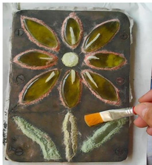
Fig. 11. Preparation of the plate-inlay assembly for thermoforming
