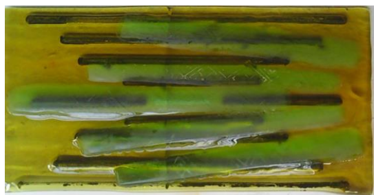
Fig. 8. Thermoformed assembly, made of brown glass, green glass, wire strands
