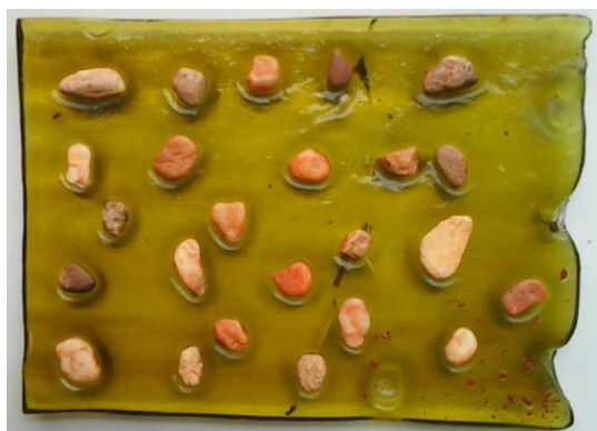
Fig. 6. Texture of the thermoformed sample, due to the shape of the pebbles
