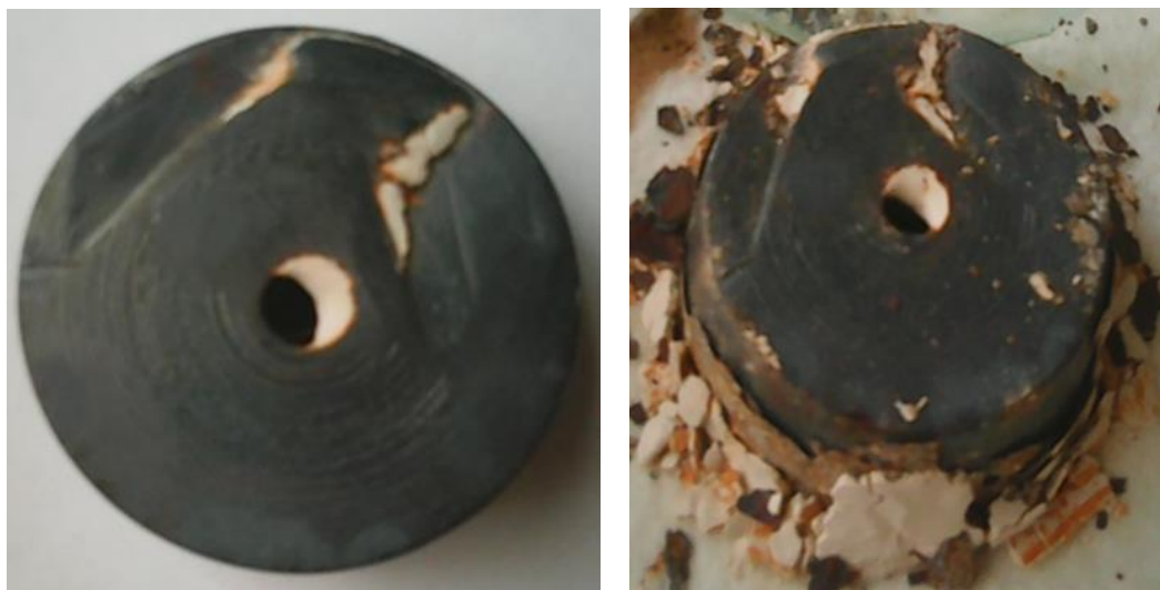
Fig. 14. Metal support for thermoforming the ashtray: a-cleaned metal support before thermoforming; b-metal support after thermoforming
