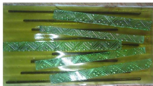
Fig. 7. The combination of the two types of glass, with different colours, placed on steel wires
