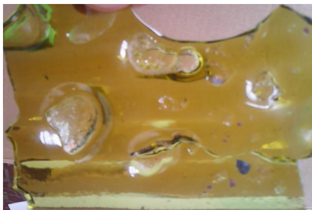
Fig. 4. Imprinting of pebbles on the surface of the piece
