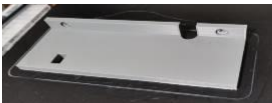
Fig. 8. The side view of the locking system 3D printed
