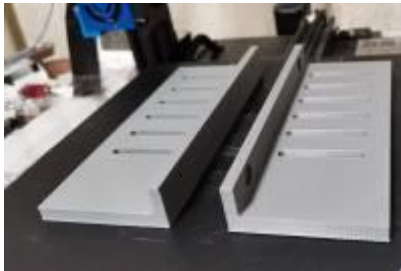
Fig. 7. The rear panel with cooling openings 3D printed PLA
