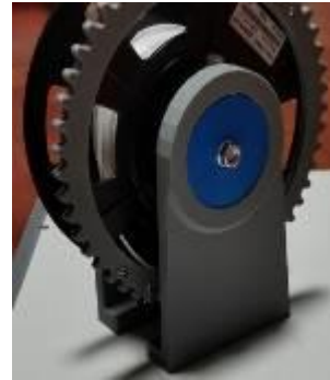
Fig. 9. 3D-printed spool holder with integrated gear ring
