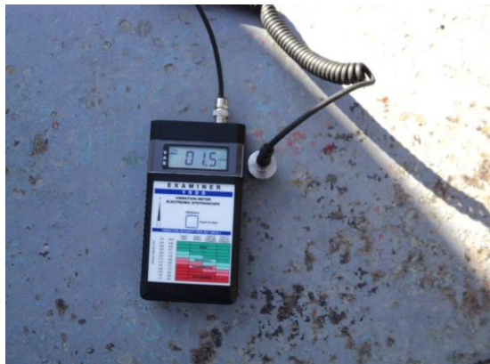
Fig. 4. Vibrations transmitted to the floor - main deck
