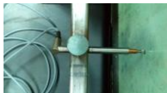
Fig. 7. Measuring device for deformation
