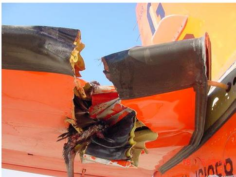
Fig. 13. A bird strike in the upper surface of the wing structure [3]
