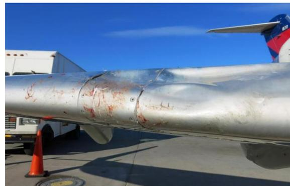
Fig. 14. A CRJ 100/200 on departure from a Minnesota airport hit a soaring bald eagle at 5000 feet AGL on March 31<sup>st</sup> 2015, causing major damage to leading edge of wing [2]
