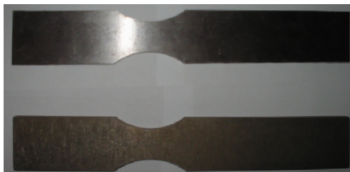
Fig. 5 The samples shape for alternating plane bending tests (nonhydrogenated – gloss and hydrogenated – mat)
