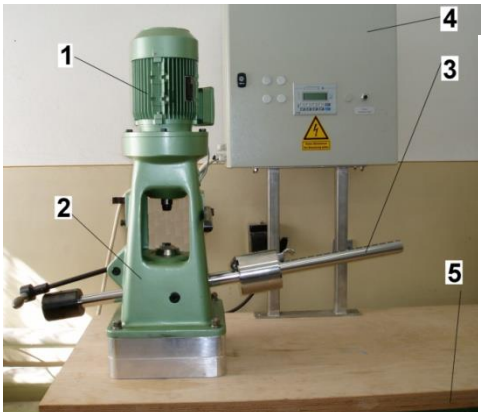
Fig. 1. The four ball machine from the oil laboratory LubriTest (without the testing system)
