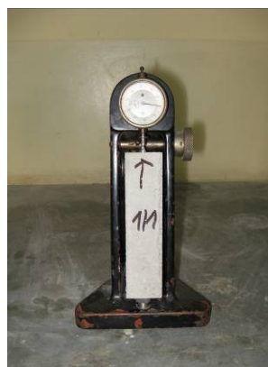
Fig. 8. Drying shrinkage measurement on a specimen with built in invar inserts
