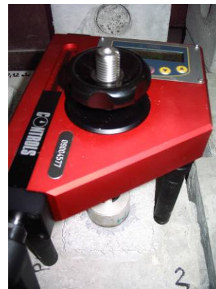
Fig. 7. Adhesion measurement using Pull off device
