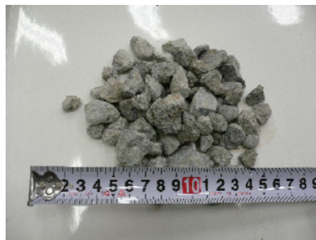
Fig. 2. Appearance of recycled concrete aggregate
