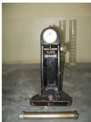
Fig. 8. Drying shrinkage measurement on a specimen with built in invar inserts
