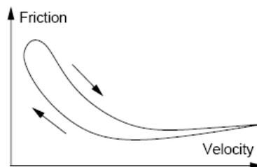
Fig. 6. The friction force versus the velocity, for a stroke
