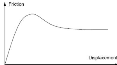
Fig. 1. The friction force evolution in a linear motion
