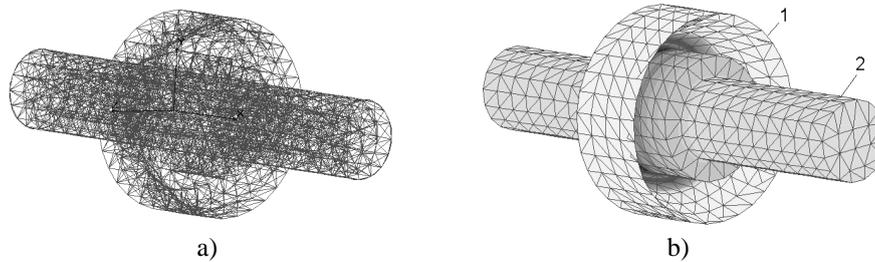
Fig. 7. The rod-lip finite element model
