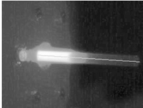
Fig. 4 A visualization of the rod thermal field as obtained with the help of a thermograph camera monitoring
