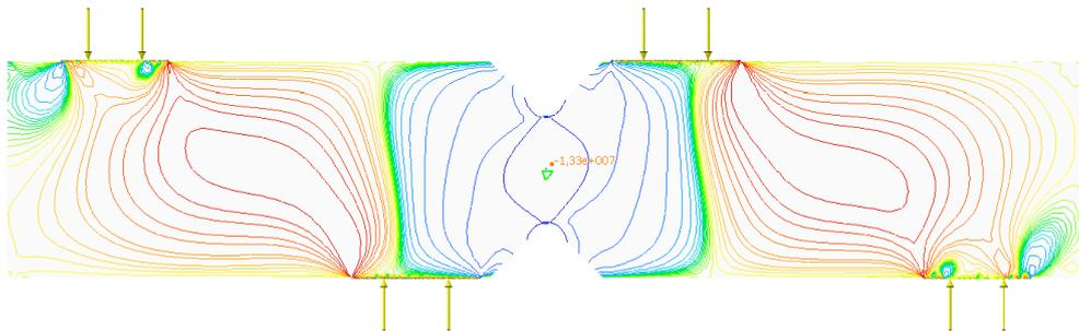
**Fig. 3.** FEA analysis of Iosipescu probe
