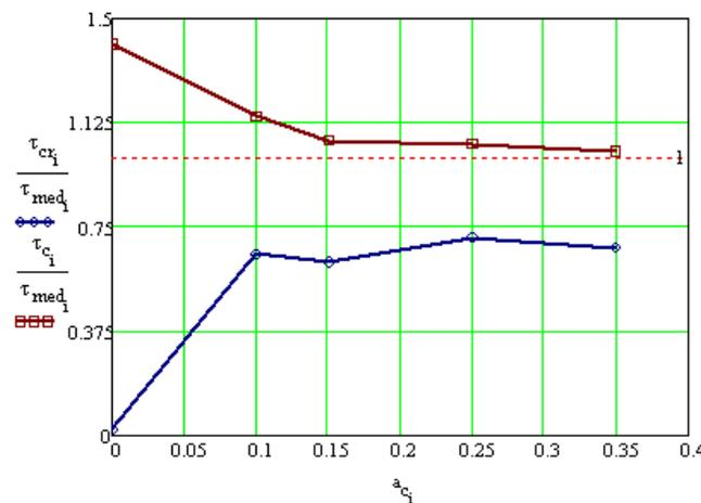
**Fig. 15.** Dimensionless stresses ( $\tau_{cr}$  - notch stress,  $\tau_c$  - central stress) versus notch depth,  $a_c$  for a notch  $\alpha = 110^\circ$
