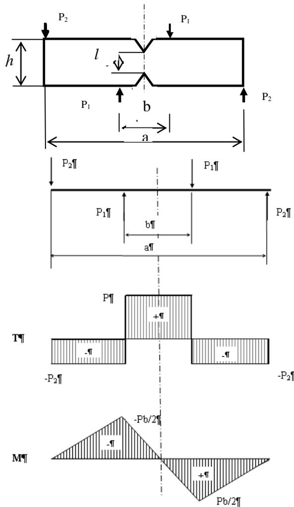
**Fig. 1.** The Iosipescu probe and the shear force (T) and bending moment (M) diagrams
