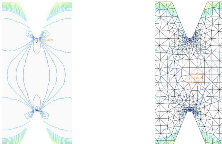
**Fig. 7.** Modified Iosipescu shear probe,  $\alpha = 45^\circ$
