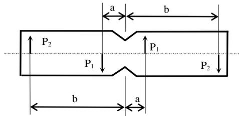
**Fig. 2.** Hawong shear test loading scheme [8]
