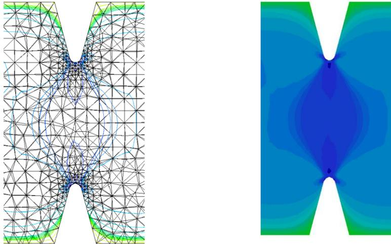
**Fig. 6.** Modified Iosipescu shear probe,  $\alpha = 30^\circ$
