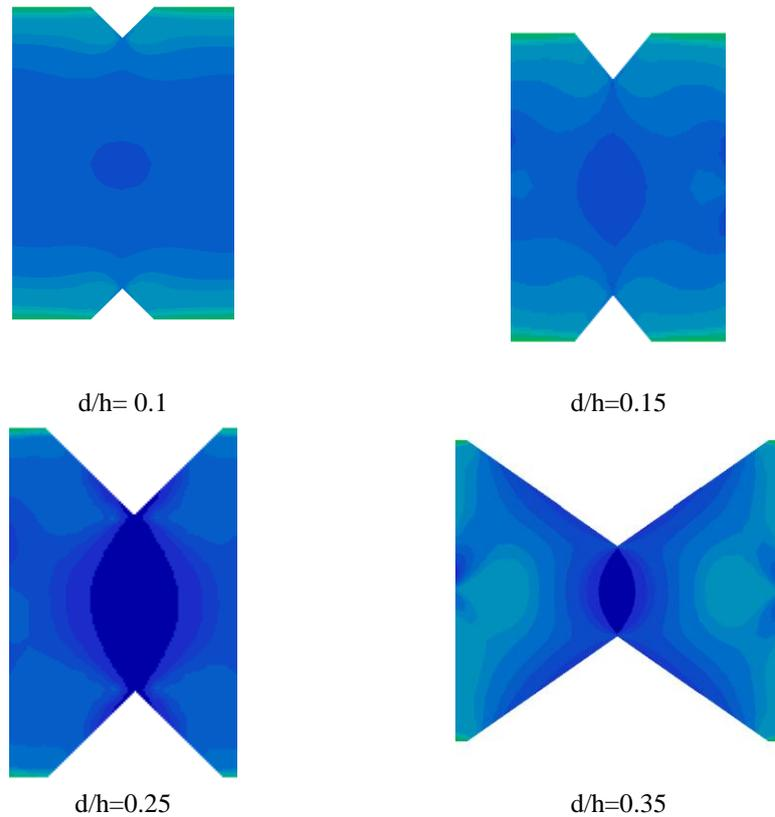
**Fig.13.** Shear stress field for different notch depths,  $\alpha = 90^\circ$
