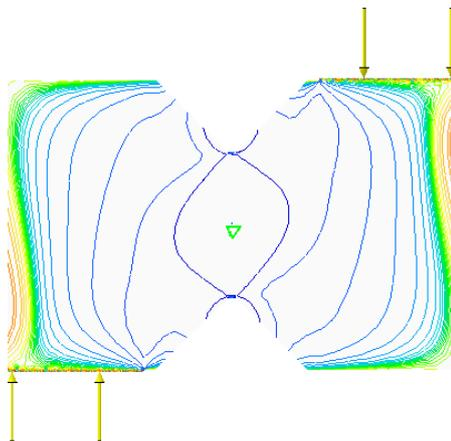
**Fig. 4.** Shear stresses contours between notches
