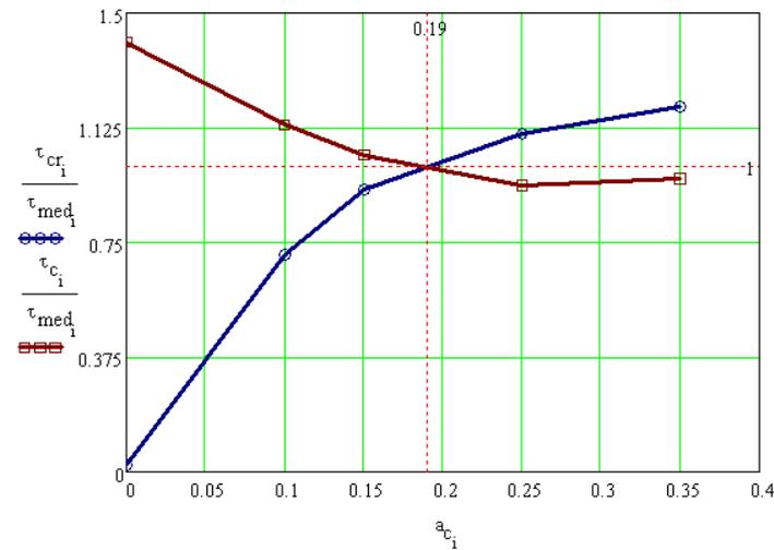
**Fig. 14.** Dimensionless stresses ( $\tau_{cr}$  - notch stress,  $\tau_c$  - central stress), versus notch depth,  $a_c$  for a notch  $\alpha = 90^\circ$
