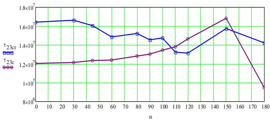
**Fig. 11.** Variation of maximum central shear stresses  $\tau_c$  and the stresses near the concentrator,  $\tau_{cr}$  with notch angle
