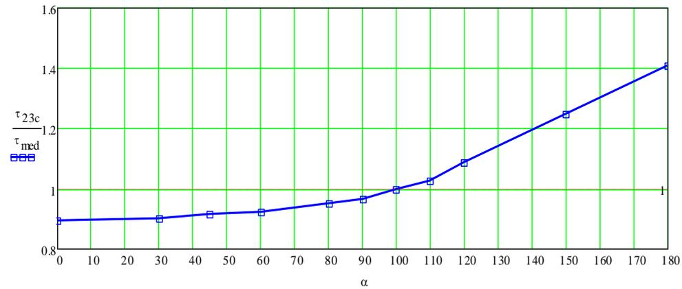
**Fig. 12.** Variation of dimensionless central shear stress with concentrator angle
