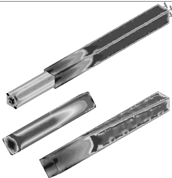
Fig. 7b. Von Mises stresses in the prismatic pair with a square cross-section
