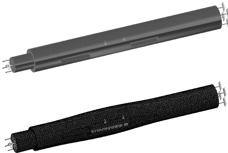
Fig. 10. Wedging assembly scheme and the deformed FEA mesh
