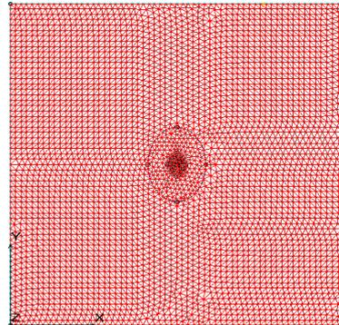
Fig. 6 Plate with single delamination
