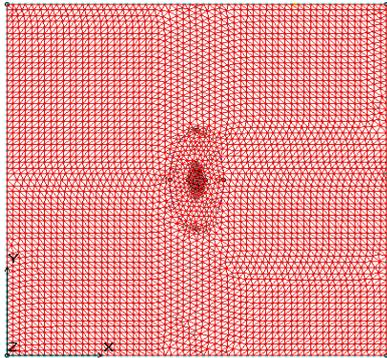
Fig. 5 Plate with single delamination
