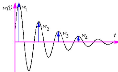
Fig. 2. The motion decay for damped vibrations
