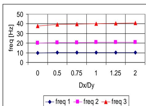
Fig. 3 The variation of the first three natural frequencies (bending vibrations) versus the diameters' ratio of the delamination area
