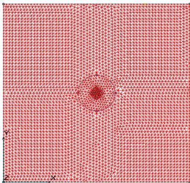
Fig. 7 Plate with single delamination
