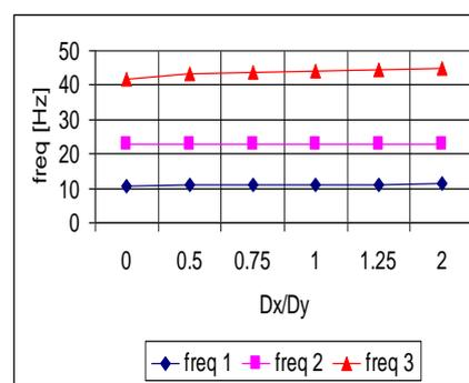
Fig. 4 The variation of the first three natural frequencies (damped bending vibrations) versus the diameters' ratio of the delamination area
