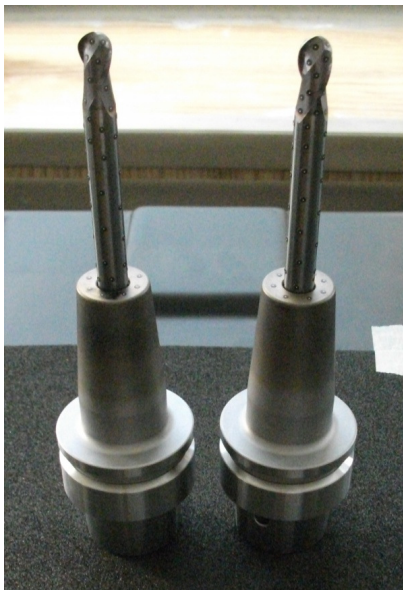
Fig. 2. The scanned ball nose end mills (lef – unused, right- used)
