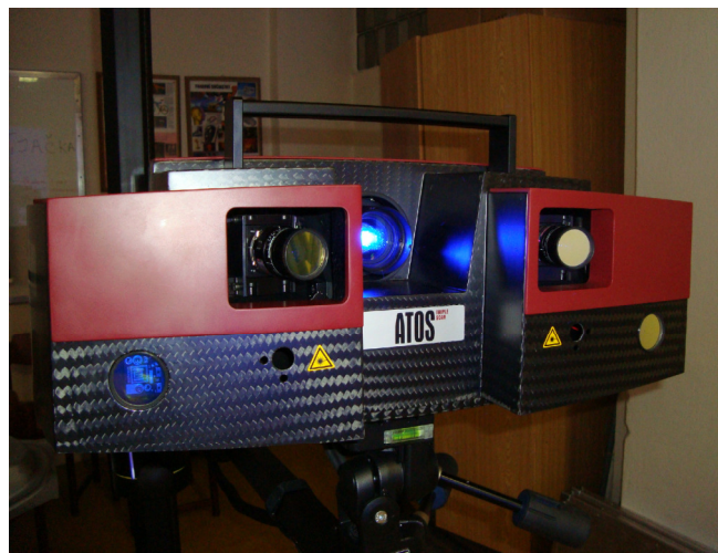
Fig. 1. The sensor (head) of optical 3D scanner GOM ATOS II SO TripleScan
