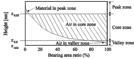
Fig. A.1. Bearing curve illustrating the calculation of  $Sbi$ ,  $Sci$  and  $Svi$
