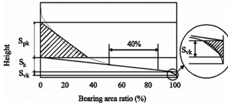
Fig. A.2. Bearing curve illustrating the calculation of  $Spk$ ,  $Sk$  and  $Svk$
