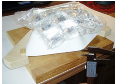
Fig. 9. Measurement of the maximal displacements of the manufactured model
