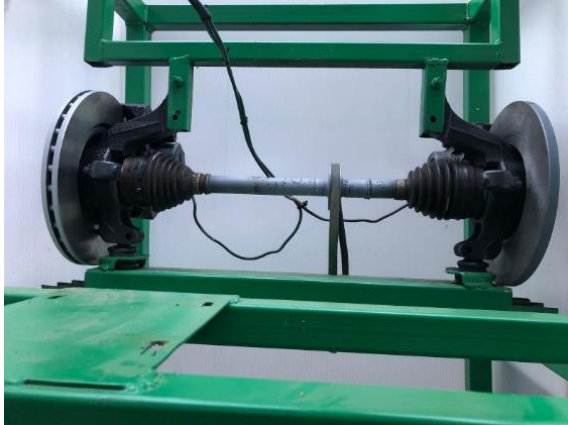
Fig. 2. Assembly of the braking system with ventilated and unventilated brake discs
