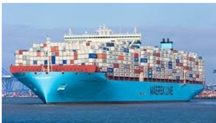
Figure 2a: Sample of the biggest ships ever built to serve global trade: Maersk Line 20,000 TEUs capacity - Year 2015
