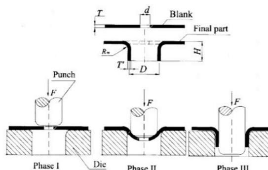
**Fig. 1.** The hole flanging process [1]
