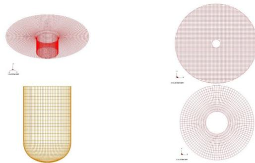
Fig. 8. Elements of hole flanging numerical model
