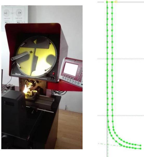
Fig. 6. The profile of the hole flanged
