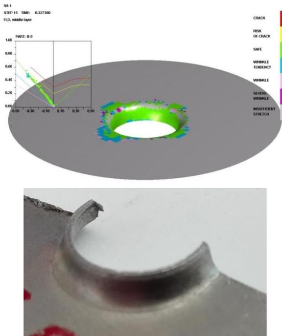
**Fig. 13.** Comparison between numerical and experimental studies for 9 mm hole diameter
