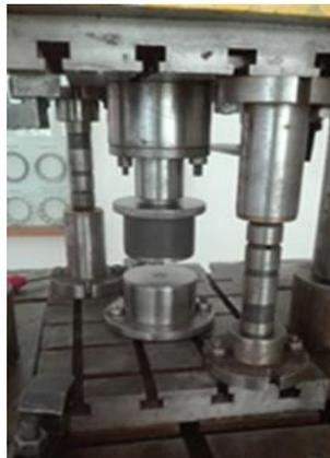
**Fig. 3.** Tool used for hole flanging
