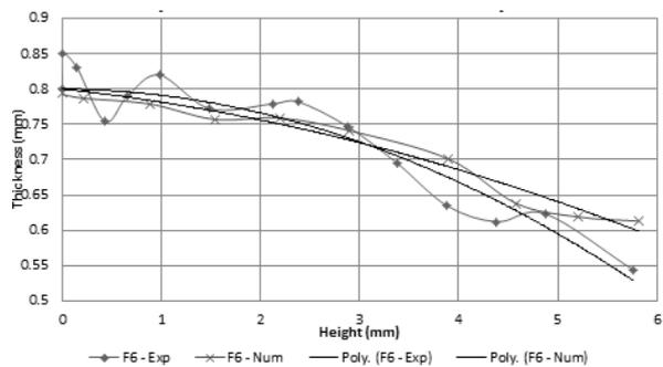
Fig. 11. Variation along the edge for a hole diameter of 6 mm and a flat punch (experimental and numerical)
