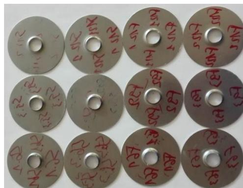
**Fig. 4.** Deformed samples with hole flanged zone
