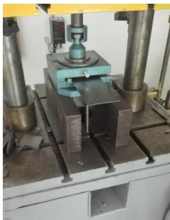
**Fig. 2.** Tool used to cut the sheet metal
