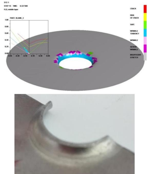
**Fig. 14.** Comparison between numerical and experimental studies for 12 mm hole diameter
