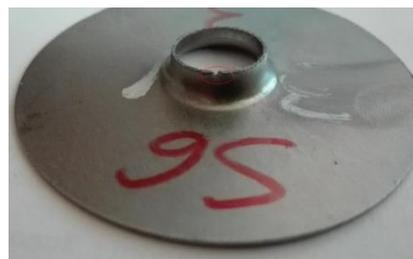
**Fig. 5.** Typical defect: a crack on the edge
