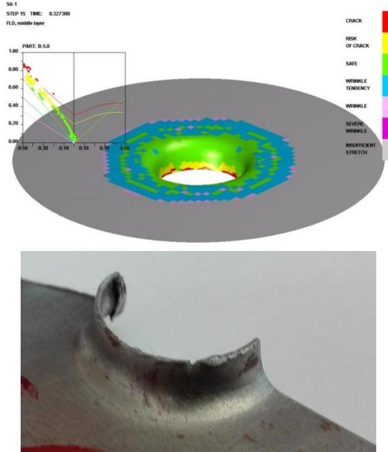
**Fig. 12.** Comparison between numerical and experimental studies for 6 mm hole diameter
