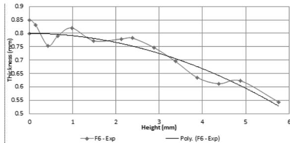
Fig. 7. Thickness variation along the edge, 6 mm inner diameter and a flat punch
