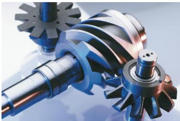
**Fig. 1.** Single screw compressor [2]
