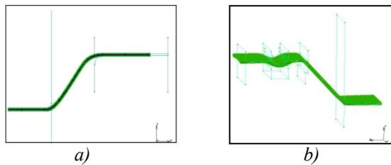
Fig. 6: Numerical model of tests: a) 2D draw bending test; b) 2D drawbead test
