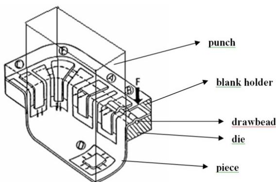
Fig.1: Complex deep drawing process [2]
