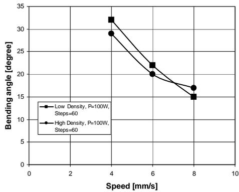
**Fig. 4.** Laser bending angle as function of the laser speed
