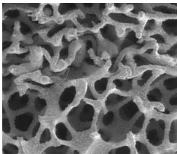
**Fig. 1.** Metal foam structure
