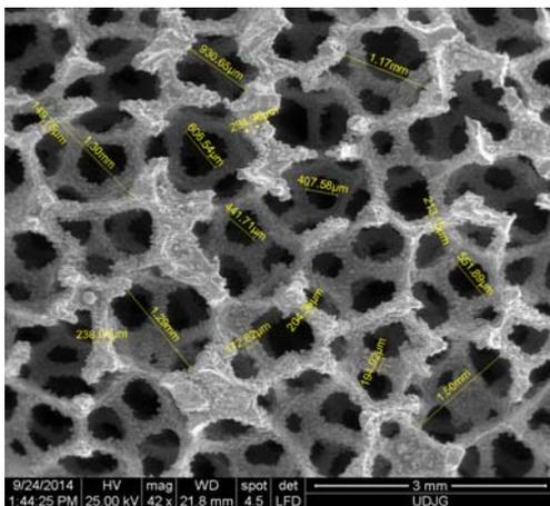
**Fig. 11.** SEM images of Al foams of higher density, laser bent with velocity 8 mm/s
