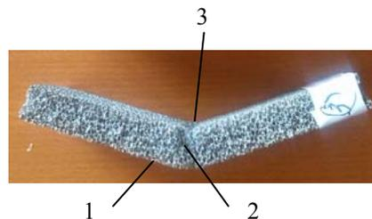
**Fig. 9.** Investigation zones in the bent foam
