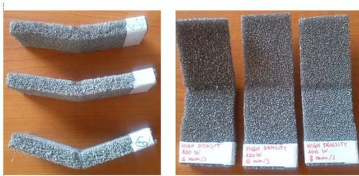
**Fig. 6.** Laser bent foams of higher density
