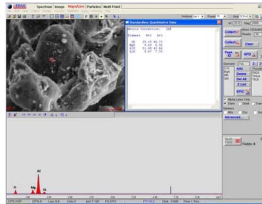
**Fig. 7.** EDX analysis of a high density foam sample, 8 mm/s scan velocity (interior zone)
