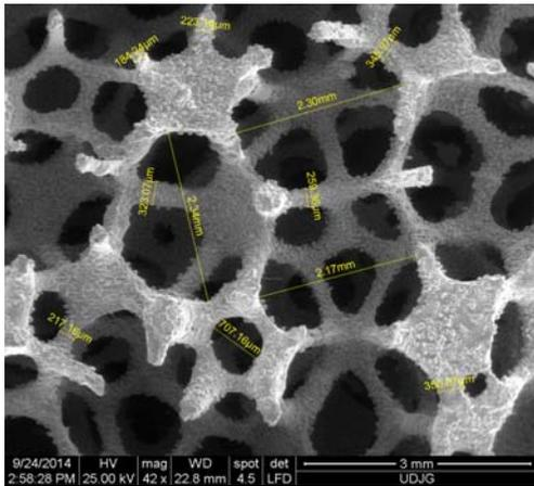
**Fig. 10.** SEM images of Al foams of lower density, laser bent with velocity of 8 mm/s
