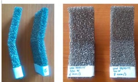
**Fig. 5.** Laser bent foams of lower density
