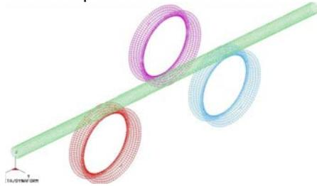
Fig. 5. Tool model used in three-roll bending process simulation
