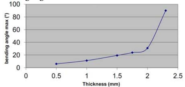
Fig. 12. Variation of the maximum bending angle reached before buckling with thickness
