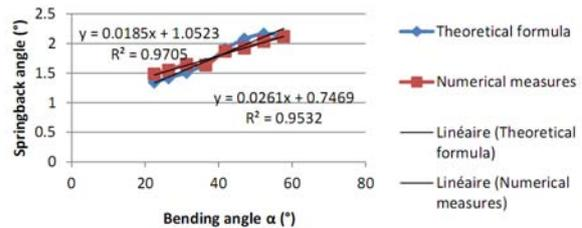
Fig. 17. Springback angle variation with the bending angle  $\alpha$ , theoretical and numerical measurements
