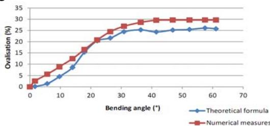
Fig. 10. Ovalization variation with bending angle for 2.3mm thicknesses
