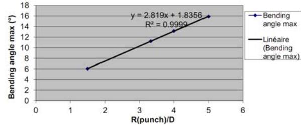
Fig. 11. Maximum bending angle reached before buckling
