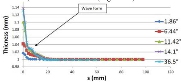
Fig. 14. Thickness variation along the tube axis for several bending angles
