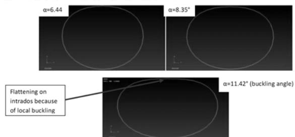
Fig. 8. Progressive ovalization of the central section leading to local buckling
