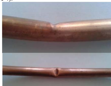
**Fig. 4.** Wrinkling of the copper tube
