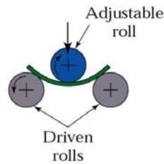
**Fig. 1.** Three-roll bending process
