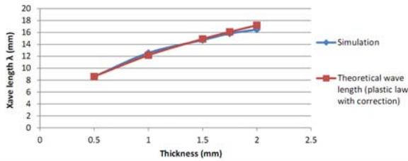
Fig. 13. Variation of the wave length with thickness
