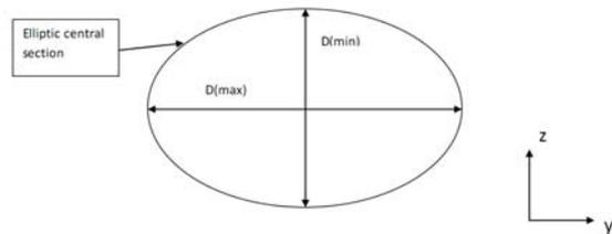
Fig. 7. Schema of the ovalized and elliptic central section
