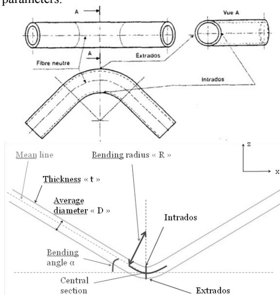
**Fig. 2.** Parameters of the deformed tube
