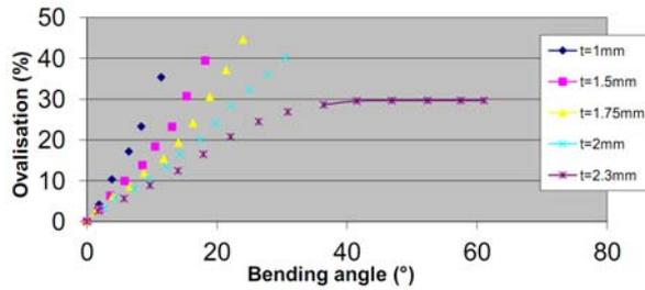
Fig. 9. Ovalization variation with bending angles for several thicknesses
