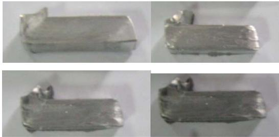
**Fig. 1. ECAP samples after 1(a), 2(b), 3(c), and 4(d) passes**
