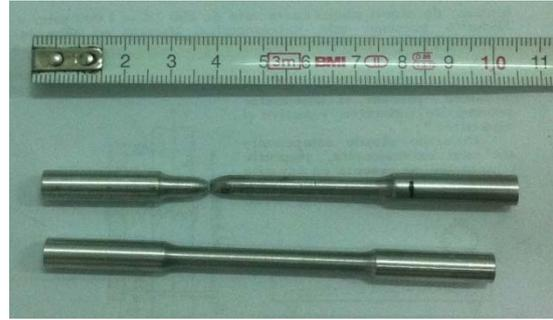
**Fig. 2. Shape of the specimen before and after the tensile test, for commercially pure A6063**
