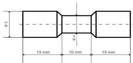
**Fig. 4. Shape and dimensions of the sub-sized specimen for tensile-test, after ECAP with 4 passes**
