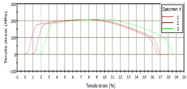
**Fig. 3. Tensile-stress-strain curves of the ‘unECAPed’ aluminium A6063**
