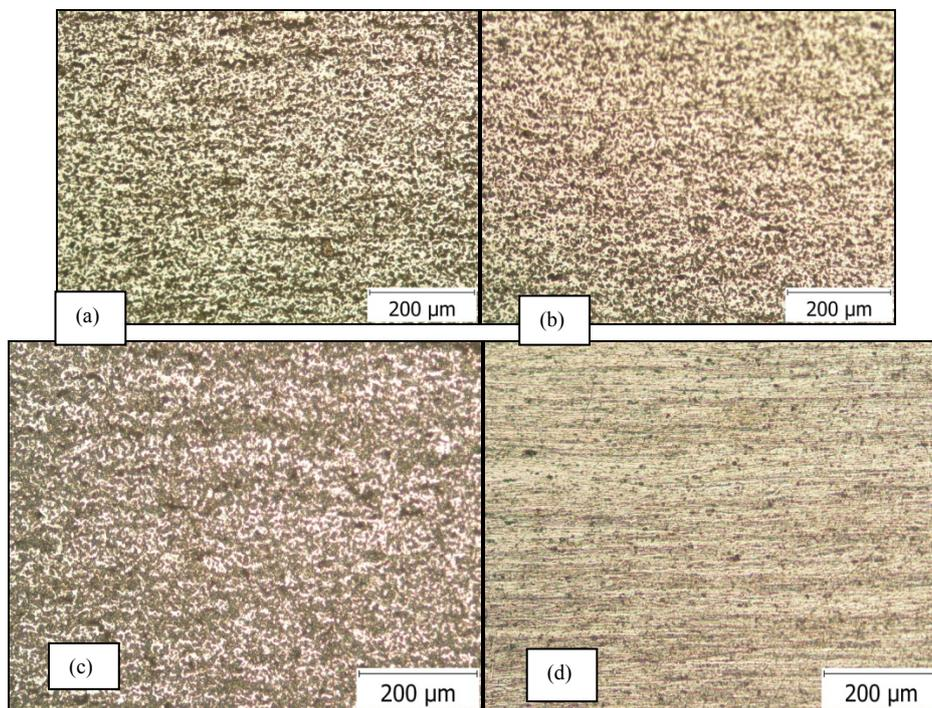
**Fig. 6.** Optical microscopy images of the aluminium surface after ECAP processing (200x) for: (a) 1 pass, (b) 2 passes, (c) 3 passes, (d) 4 passes
