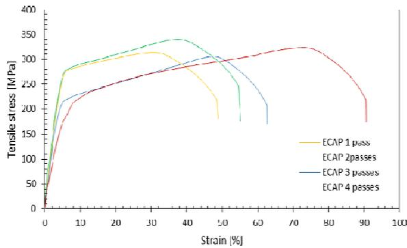
**Fig. 5.** Tensile stress-strain curves for each ECAP pass sample
