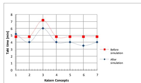
Fig. 4. Takt time variations for each concept before and after the simulation process
