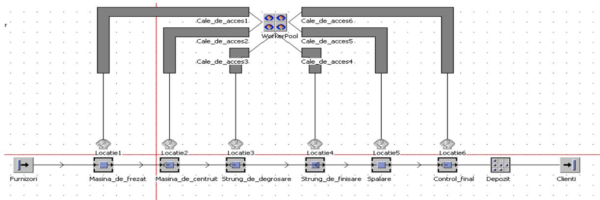
Fig. 2. Model created for the simulation process before applying Kaizen concepts
